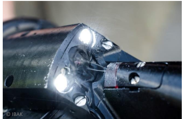
Rinsing process of camera lens of the milling robot Nanogator
